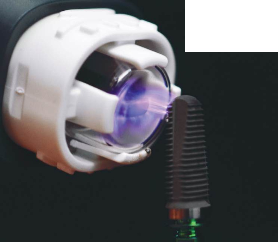
PiezoBrush PZ3 for handheld plasma surface treatment
