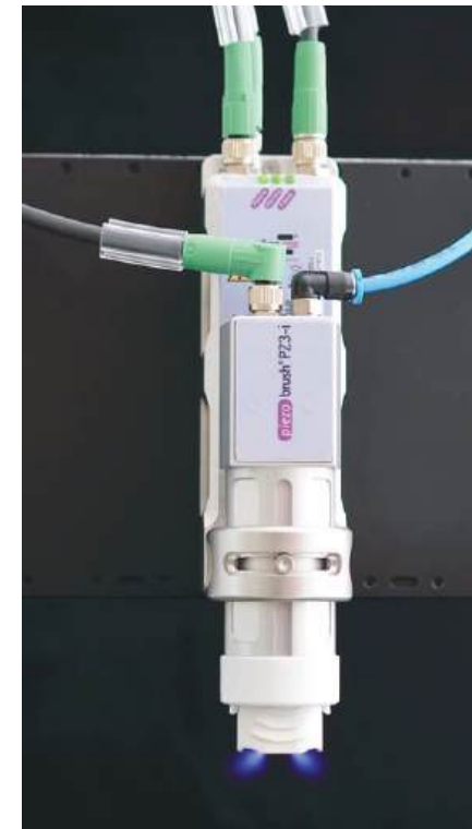
PiezoBrush PZ3-i for semi-automated or automated plasma surface treatment
