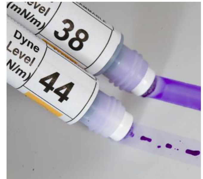
Dyne Test Pens for surface energy measurement
