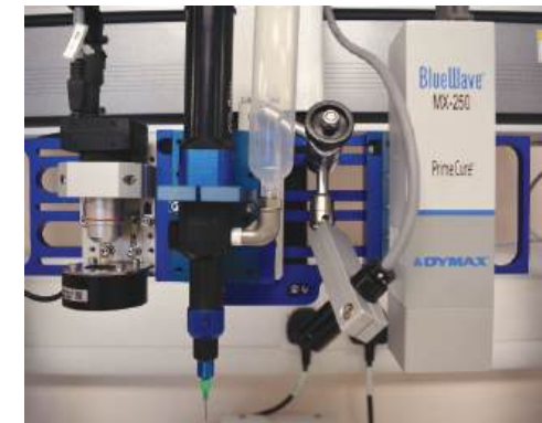
Dispensing robot with vision and UV curing
