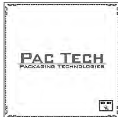
Die size: 10x10mm (394mils sq) Pitch: 100µm (3.94mil)
