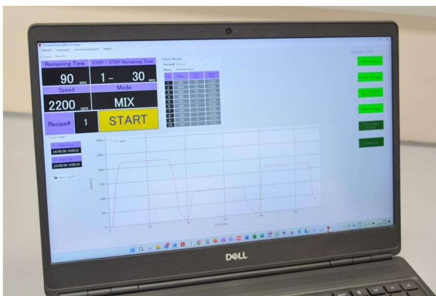
Figure 2 – THINKY ARE-312 mixer process data being recorded by remote software
