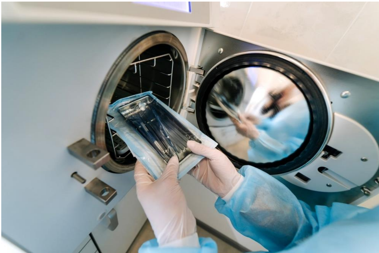
Figure 5 – Autoclaving or steam sterilisation is a very challenging process for an adhesive to withstand
