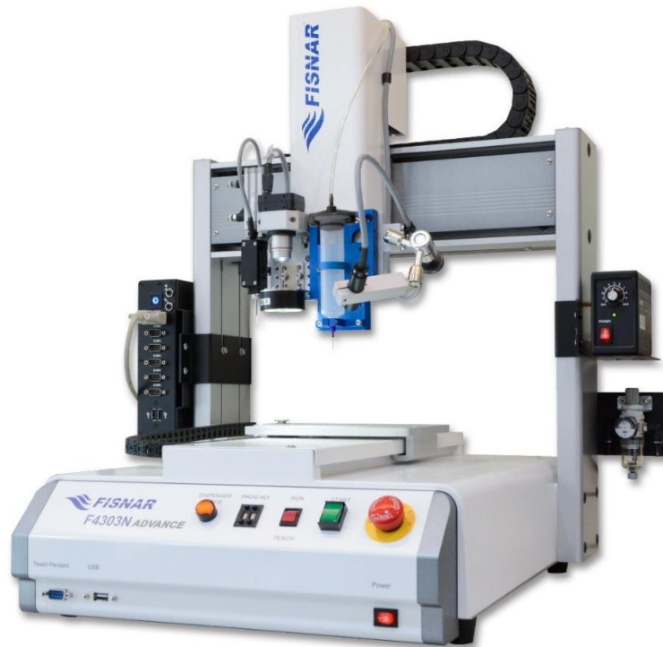
Figure 3 – Fisnar dispensing robots enable the accurate and repeatable application of materials during production
