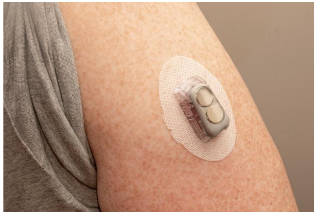
Figure 1 – Medical device adhesives can be used to bond components within glucose or electrocardiogram (ECG) monitors
