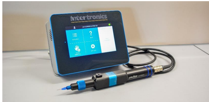
Figure 7 – A progressive cavity pump in a format suitable for integrating into a production process
