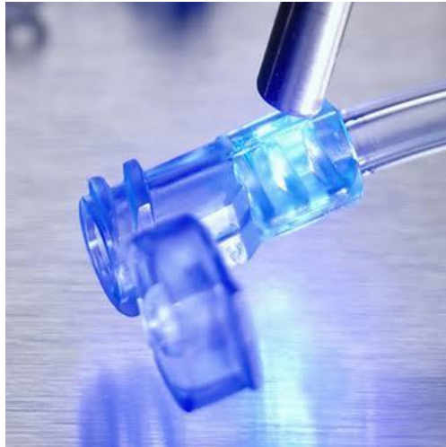
Figure 1 – A single part adhesive curable with UV LED light reduces process variables in medical device bonding
